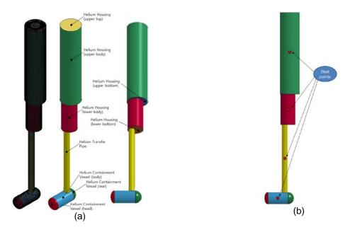
Figure 5 Finite element model and blast points for the simulations
