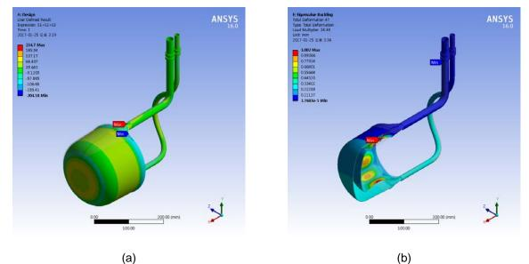
Figure 11 The sum of principal stress and buckling mode of the moderator cell
