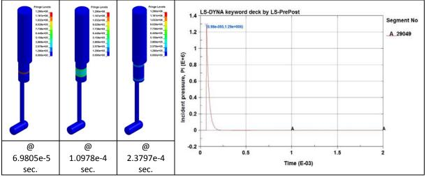
Figure 7 Incident pressure wave contour and history plot (helium housing lower)
