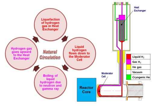
Figure 1 Schematic drawing of thermo-siphon
