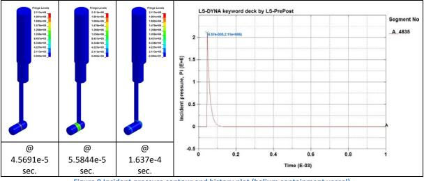
Figure 9 Incident pressure contour and history plot (helium containment vessel)
