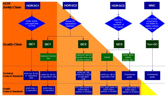
Figure 4 Safety Class, Quality Class, and Codes and Standards for OYSTER Project
