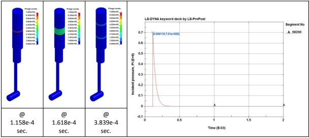
Figure 6 Incident pressure wave contour and history plot (helium housing upper)
