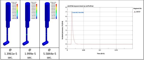
Figure 8 Incident pressure wave contour and history plot (helium transfer pipe)
