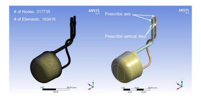
Figure 10 Finite element model for moderator cell
