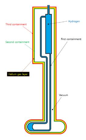
Figure 2 Triple containment design concept
